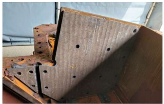
6. Opening Cover 초경 Liner 취부
