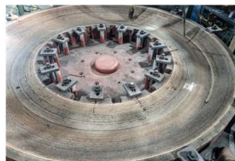
21. BULLRING SEGMENT 육성용접완료
