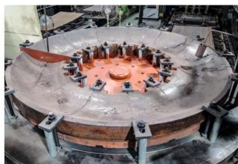
19. BULLRING SEGMENT 육성용접준비
