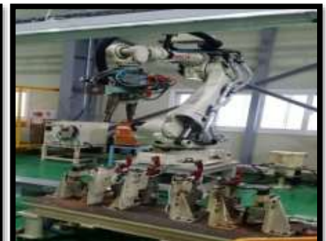
Robot Spot Welding Line
