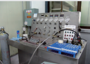
Valve Test Snad 350kg/cm 2 , 80Lpm
