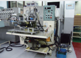
Valve Test Snad 210kg/cm 2 , 20Lpm
