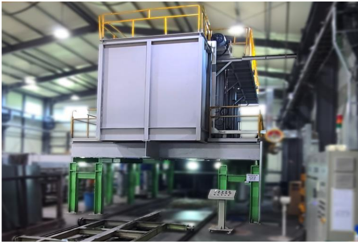
Solution Furnace (1) 1.8m(W) X 1.6m(H) X 7.5m(L)
