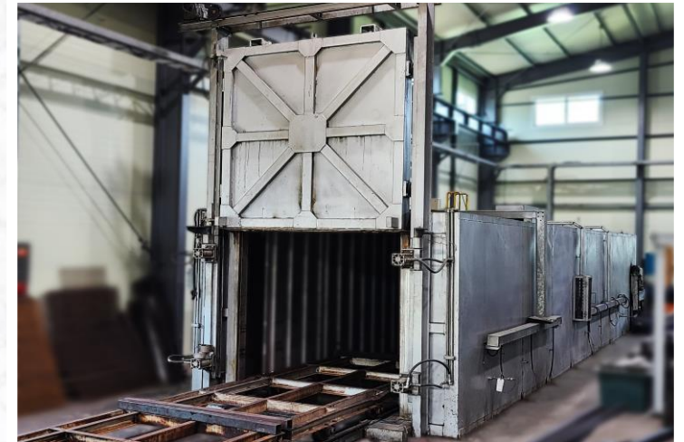
Aging Furnace 1.8m(W) X 1.6m(H) X 10.5m(L)
