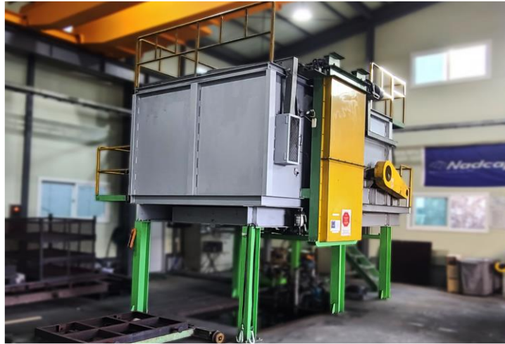
Solution Furnace (2) 1.0m(W) X 1.0m(H) X 1.5m(L)
